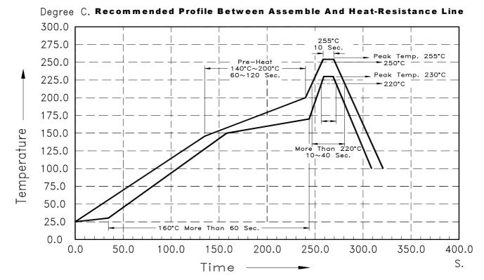
The Profile is available that must to use SnAg  $_{\left(x=3.3\sim3.8\right)}$  Cu  $_{\left(y=0.2\sim0.7\right)}$  solder paste
